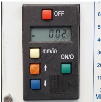
Digital Readout On Quill Depth
