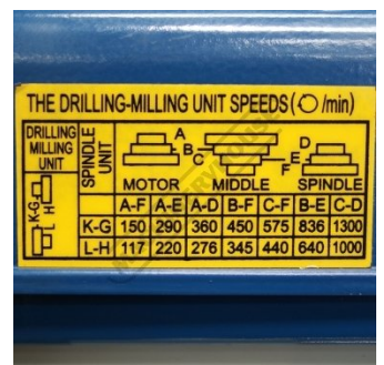
Drill Mill Spindle Speeds
